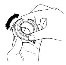
Replace the bearing with a new one if there is excessive play.
